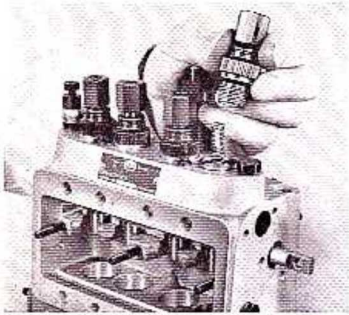
FIG. 9. REMOVING THE DELIVERY VALVE HOLDERS
